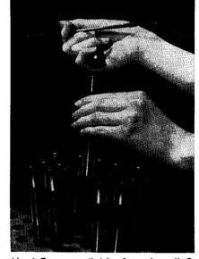
Alumi-Caps available from Lowell S. Fisher Co. made of lightweight aluminum for protection of culture tubes from contamination by air carried dust. The caps can be made to fit any size culture tube and are available in natural aluminum or anodized in red, blue, green, or yellow. The caps can be heat sterilized and reused **PE3**
